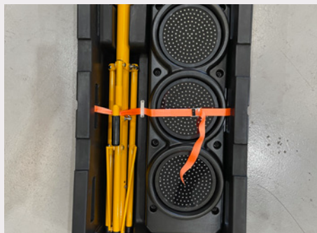
Loop the webbing strap through the cam buckle and tighten, taking care not to over-tighten or scratch signal aspects.
