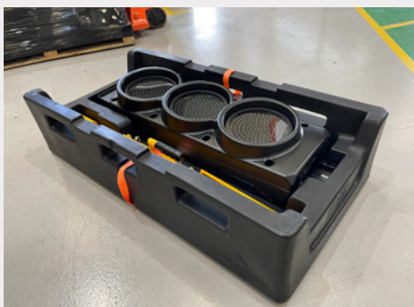
Carefully place the signal head face up in the stillage, bottom first to protect the radar and antenna.
