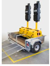
Repeat for remaining signals. If carrying two signals, arrange diagonally across the trailer bed to balance the load.
