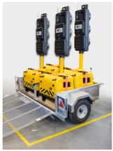
Once signals are loaded, raise the ramp and secure with the antiluce pin.
