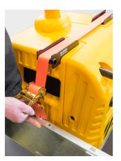
Secure signals using ratchet straps, fastened to the trailer eyelets and positioned across the provided tie-down points.
