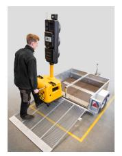
Ensure trailer is on a level surface and connected to a suitable tow vehicle, lower ramp and carefully load signal.
