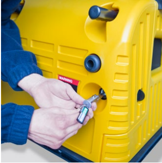
Unlock the battery secure bar.
