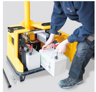
And easily removed by the integral handles. Reverse the procedure to re-install.
