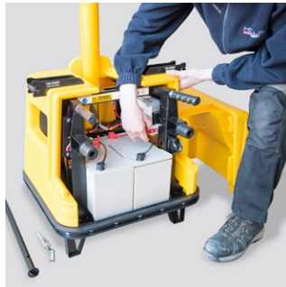
The batteries can now be unplugged.
