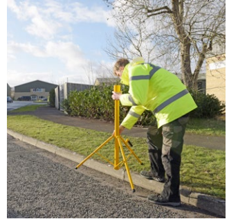
Legs deploy and catch locates at base of stand.
