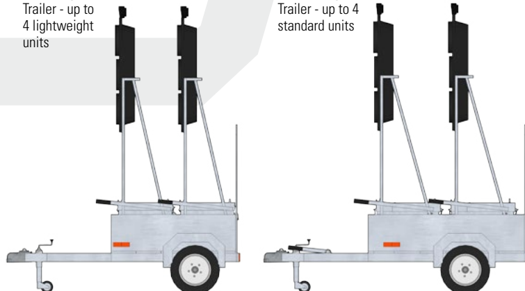
Both Trailers have adjustable jockey wheels for easy manoeuvrability
