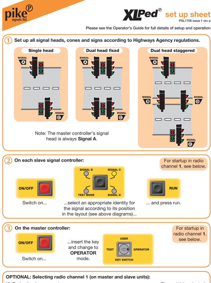
XL Ped units always revert to radio channel **2**. For layouts that have two crossings, one XL Ped set must use radio channel **1**.
