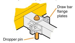
Note: Earlier models use flange plates with two bolts instead of the four shown above.
