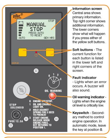
For details about how to configure the signals, please refer to the set up sheets and user guides: XL 2 Phase - PSL1654 (sheet) or PSL1648 (guide) XL Multiphase - PSL1569 (sheet) or PSL1573 (guide)
